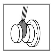
**6.** Pull the broken cap off and then peel off the filter and diffusive gel layer to reveal the bottom binding-gel layer.
