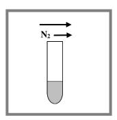
**9.** Evaporate the eluant under a gentle stream of nitrogen to near dryness.
