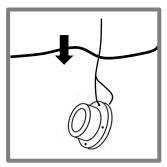
**3.** Ensure that the white window face of the DGT unit is fully immersed during the deployment period.
