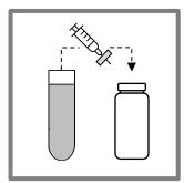
**10.** Re-dissolve with 1 mL methanol. Filter the solution through an 0.22 μm syringe filter to an amber vial.
