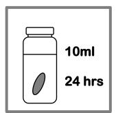
**7.** Fully immerse the resin gels in 10 mL MeOH containing 0.5% NH<sub>3</sub>. Leave for at least 24 hours before analysis.
