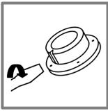
**5.** To retrieve the resin gel after deployment, insert a suitable screw driver into the groove in the cap and twist it. The cap will be broken at the weak point.
