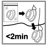
1. Having placed the DGT unit in its deployment holder or simply attached it to any deployment device by tying it with a pre-cleaned fishing line threaded through the hole on the rim of the unit, deploy the unit immediately (minutes).
