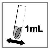
2. Extracte the resin gel with 1 mL 6 M HNO<sub>3</sub> in a glass vial for 6 hours at 70 °C.
