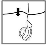
**3.** Ensure that the white face of the DGT unit is fully immersed during the deployment period. Provide an accurate record to the nearest minute of the deployment time
