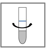
**10.** Centrifuge the eluate at 3000 rpm for 10 min, then keep the supernatant for further analysis using for example GC-AFS (in this case, ethylation of the supernatant is necessary).
