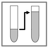
8. Remove the binding layer from the tube, squeezing out any residual liquid. Then dilute the eluate by adding 9 mL of MilliQ water (depending on the concentration levels of Hg) prior to analysis using Cold-Vapor AFS or ICPMS.
