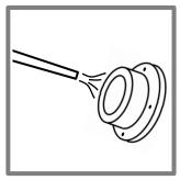
1. After retrieving the DGT device from the deployment environment thoroughly rinse the DGT device with ultrapure water.
