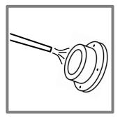
1. After retrieving the DGT device from the deployment environment thoroughly rinse the DGT device with ultrapure water.
