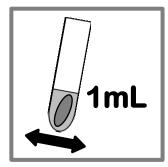
**7a.** For urgent analysis, agitate the tube containg the binding gel and 1 ml of 1.0 M HCl on a shaker.
