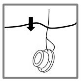
**3.** Ensure that the white face of the DGT unit is fully immersed during the deployment period.
