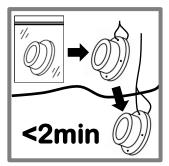
1. Having placed the DGT unit in its deployment holder or simply attached it to any deployment device by tying it with a fishing line threaded through the hole on the rim of the unit, deploy the unit immediately (minutes).
