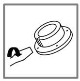
5. To retrieve the resin gel after deployment, insert a suitable screwdriver into the groove in the cap and twist. The cap will be broken at the weak point. If this fails, using clean tweezers break the white filter membrane and pull out the gels. The binding gel is the lower one.
