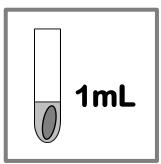
7. Place the binding gel in a clean sample tube and add 1 ml of 1.0 M high purity HNO<sub>3</sub> solution.
