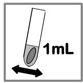
**7a.** For urgent analysis, agitate the sample tubes containing either nitric acid or sodium hydroxide on a shaker.
