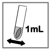
**7a.** For urgent analysis, agitate the tube containing the binding gel and 1 ml of 1.0 M HCl on a shaker.
