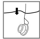
**3.** Ensure that the white face of the DGT unit is fully immersed during the deployment period.
