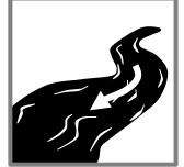
2 Ensure the DGT device is deployed in flowing (or moving) water, but avoid excessive turbulence, particularly bubbles. Large open waters including lakes usually have sufficient natural flow through wave action.
