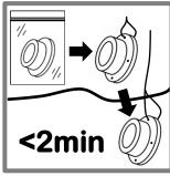
1. Having placed the DGT unit in its deployment holder or simply attached it to any deployment device by tying it with a fishing line threaded through the hole on the rim of the unit, deploy the unit immediately (minutes).
