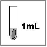
7. Place the binding layer (or sliced portion of it for sediment probes)in 5 ml of high purity water for 1 hour. Then place it in a clean sample tube and add 1 ml of 1.0 M high purity HCl.
