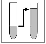
**9.** Dilute, as necessary for analysis using ultrapure water (18.2MOhms).
