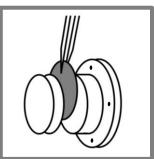
**6.** Remove the broken cap and then peel off the filter and diffusive gel layer to reveal the bottom binding-gel layer.
