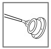
1. After retrieving the DGT device from the deployment environment thoroughly rinse the DGT device with ultrapure water from a wash bottle.
