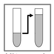
**9.** Dilute, as necessary for analysis using ultrapure water (18.2MOhms).
