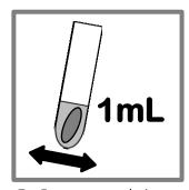
**7a.** For urgent analysis, agitate the tube containing the binding gel and 1 ml of 1.0 M HCl on a shaker.
