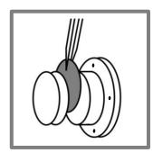
**6.** Remove the broken cap and then peel off the filter and diffusive gel layer to reveal the bottom binding-gel layer.
