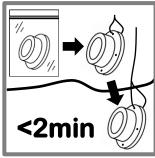
1. Having placed the DGT device in its deployment holder or simply attached it to any deployment device by tying it with a fishing line threaded through the hole on the rim of the unit, deploy the unit immediately (minutes).
