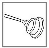
**1.** After retrieving the DGT device from the deployment environment thoroughly rinse it with ultrapure water.
