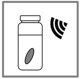
8. Make sure the resin gel is fully immersed in the methanol solution. Ultrasonic bath for 30 minutes. Remove the resin gel. (Recommend)
