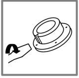
**5.** To retrieve the resin gel after deployment, insert a suitable screw driver into the groove in the cap and twist it. The cap will be broken at the weak point.
