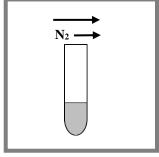
**10.** Evaporate the eluant under a gentle stream of nitrogen to near dryness.
