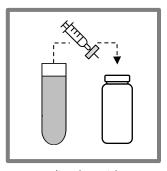
**11.** Re-dissolve with 1 mL methanol. Filter the solution with 0.22μm syringe filter to an amber vials.
