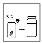
9. For NCBs, add 5mL tolunen, then ultrasonic bath for 30 min. Transfer the eluent to a new vial. Repeat the extraction one more time. Remove the resin gel and mix the two eluants in the new vial.
