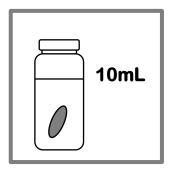
7. Place the resin gel in a clean amber glass vial and add 7 ml methanol and 3 ml 1M NaOH.
