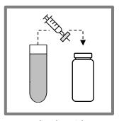
11. Re-dissolve with 1 mL methanol. Filter the solution with  $0.22\mu m$  syringe filter to an amber vials.
