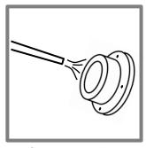
1. After retrieving the DGT device from the deployment environment thoroughly rinse it with ultrapure water.
